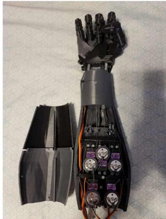
The prosthetic arm has five servo motors in the forearm compartment that control each finger. There is also a servo in the below the wrist which controls the wrist.
